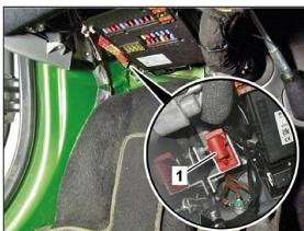
The high-voltage disconnect device is located on the underside of the instrument panel on the left side.
