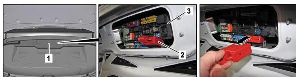
The high-voltage disconnect device is located under the lid of the fuse and relay box on the rear panel in the boot.
