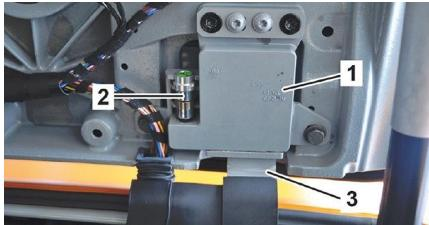
The SLS AMG is equipped with a safety system which uncouples the door hinges from the hinge arms when the vehicle comes to rest lying on its roof after an accident. Each door hinge (1) contains a pyrotechnic initiator (2) which is triggered by the restraint systems control unit. When the door lock is opened, the doors can be pulled off the hinge arms (3).
