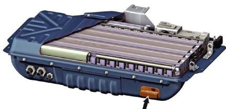
The high-voltage disconnect device is located on the right at the rear of the high-voltage battery.
