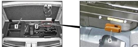
Lift load compartment floor (1) / Remove cover (2) / Push switch (3) to the right and pull off high-voltage battery
