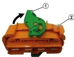
The high-voltage disconnect device is located on the underside of the high-voltage battery on the right at the rear.
