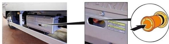
The EMERGENCY OFF button is located in the cutout in the side panel of the high-voltage battery.
