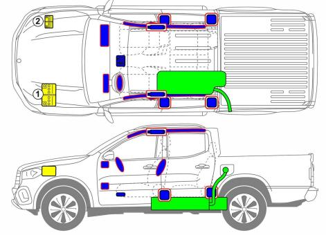
① On-board electrical system battery
