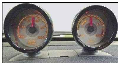
⑤ High-voltage battery state of charge (SOC) and power flow display device
