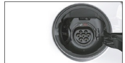
③ HV charge socket ECE
