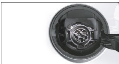
④ HV charge socket USA/Canada
