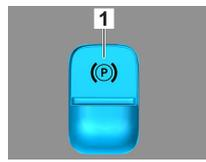
Press the P switch on the gear selector (1). The parking brake is automatically activated.
