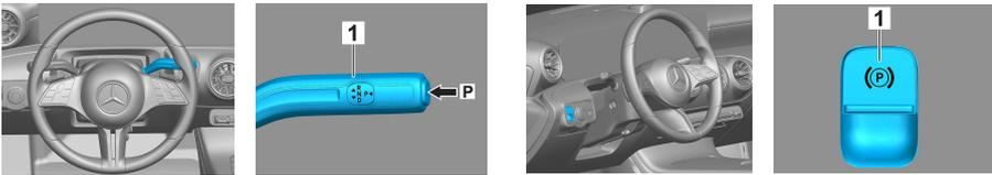
Press the P switch on the gear selector (1). The parking brake is automatically activated. Electric parking brake (1)
