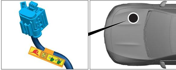
The high-voltage disconnect is located in the engine compartment on the passenger side.
