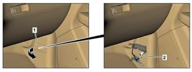
Remove cover (1) of fuse box / Cut line at marked location (2)
