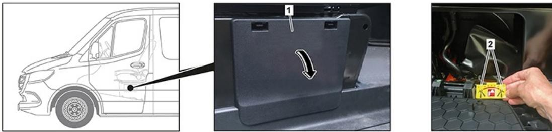
Remove the cover (1). Cut the cable at the marked point (2).
