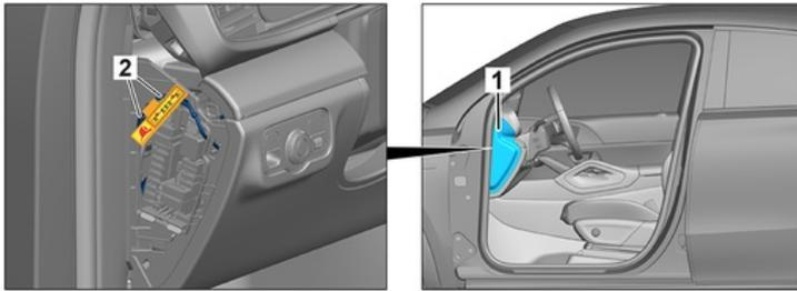
Remove the cover (1). Cut the cable at the marked point (2).
