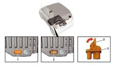
The high-voltage disconnect device is located on the underside of the high-voltage battery on the left at the rear.
