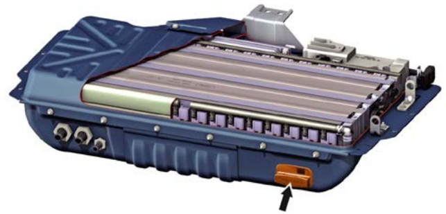
High-voltage disconnect device
