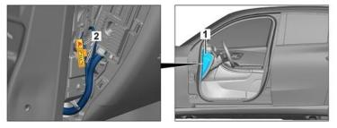
Remove the cover (1). Cut the cable at the marked point (2).
