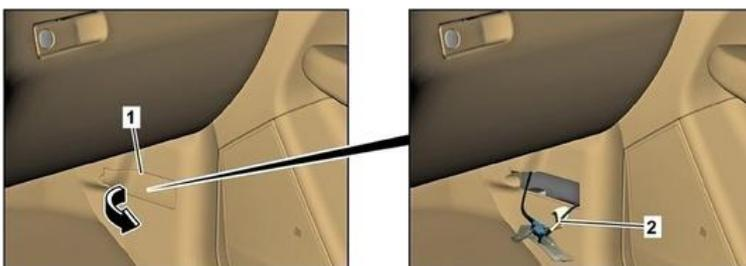
Remove cover (1) of fuse box / Cut line at marked location (2)
