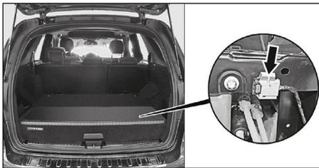
The high-voltage disconnect device is located in the trunk under the cover of the high-voltage battery.
